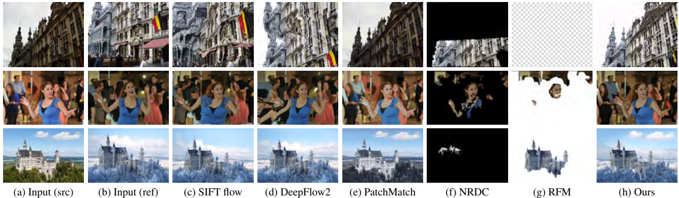
Figure 10: Comparison of different dense correspondence methods on input pairs with the same scene but large variations in view, color, and tone. (For the first example, both public result and implementation of RFM are unavailable, so we have to make the result empty here.)
