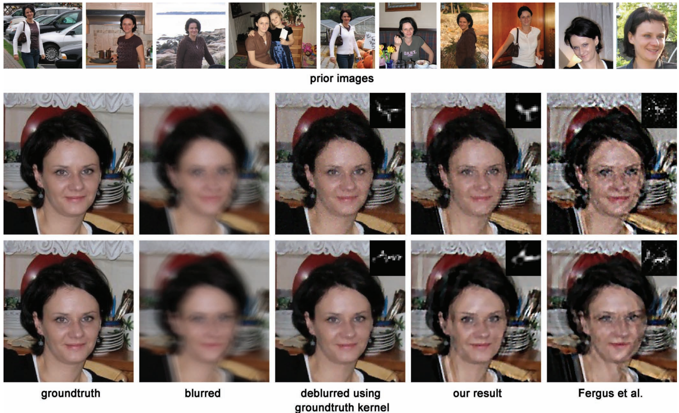
Fig. 13. Synthetic deblurring experiments. We blurred a sharp image with two different blur kernels and added 0.5% noise (second column), and then solved for the PSF using our deblurring method and the method of Fergus et al. We then deconvolved the blurred image with the ground-truth kernel (third column), our recovered kernel (fourth column), and the kernel resulting from running Fergus et al.’s code (fifth column). Each kernel is shown in the top right corner of each image.
