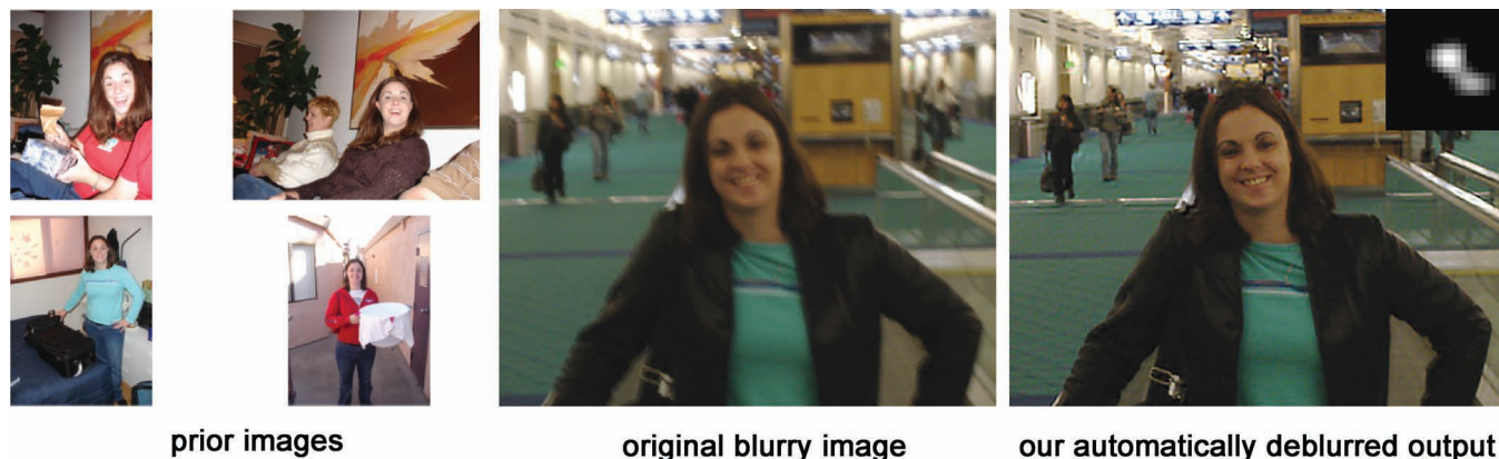
Fig. 1. Automatically correcting personal photos. We automatically enhance images using prior examples of “good” photos of a person. Here we deblur a blurry photo of a person where the blur is unknown. Using a set of other sharp images of the same person as priors (left), we automatically solve for the unknown blur kernel and deblur the original photo (middle) to produce a sharp image (right); the recovered blur kernel is shown in the top right enlarged 3\times .
