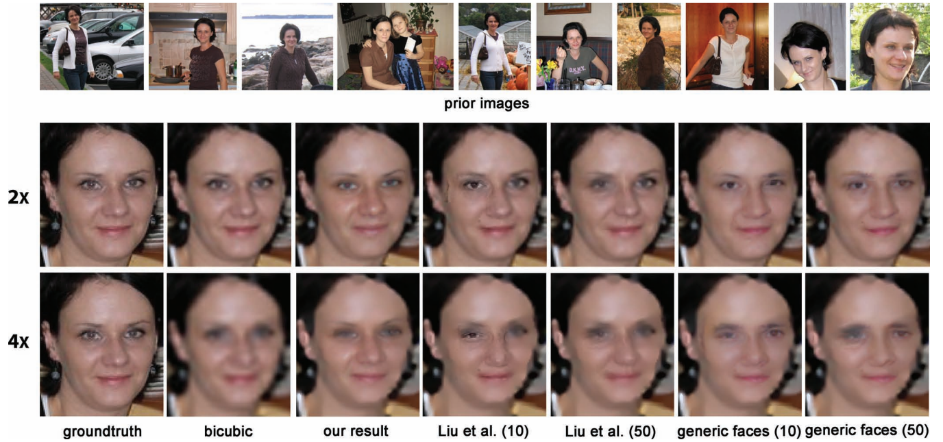
Fig. 14. Synthetic upsampling experiments. We down-sampled a sharp image by 2\times and 4\times and then up-sampled those images by 2\times and 4\times , respectively, using bicubic upsampling (second column), our enhancement algorithm (third column), an implementation of Liu et al.'s method (fourth and fifth columns), and our enhancement algorithm with a set of (the 10 and 50 best matching) generic faces (six and seventh columns).
