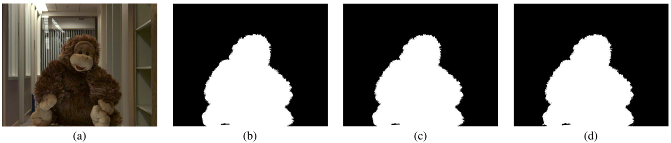
Figure 6: Varying the number of images used. (a) Central image. (b) Alpha matte using 120 images, (c) 60 images, and (d) 8 images.
