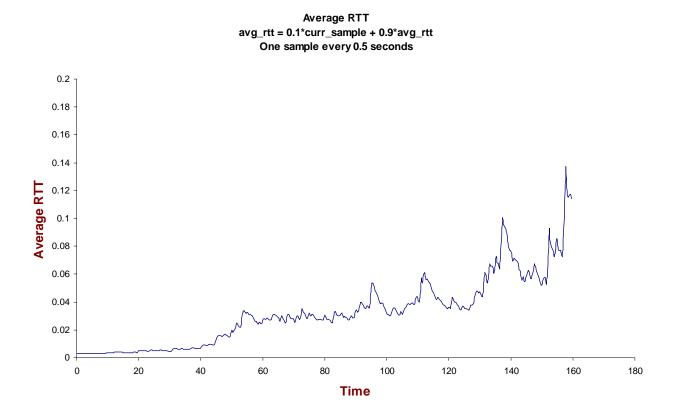
A new 100Kbps CBR connection starts every 10 seconds, between a new pair of nodes. All nodes hear each other.
