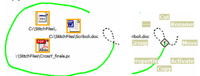
Fig. 13. Animated stroke extension (see also our video). Left: Stroke extension shows how to draw a pigtail. Right: The menu pops up when the animation finishes.
