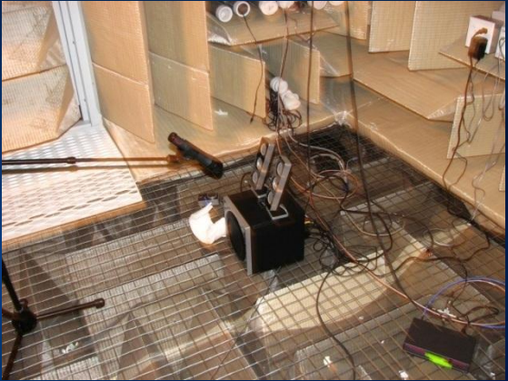
Microphone testing in Anechoic Chamber
