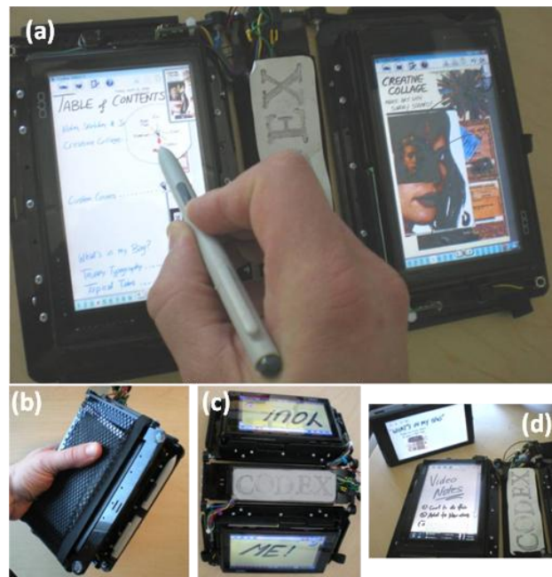
Fig. 1. Codex dual-display tablet. (a) The book posture. (b) Codex folded up for mobility. (c) Face-to-face collaboration. (d) The displays detach.
