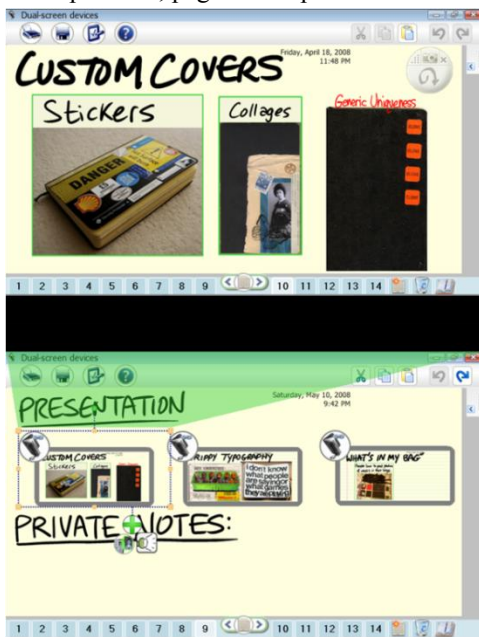
Fig. 7. Previewing a page link with the screens in landscape orientation. Selecting a link on the bottom page previews the linked page on the top screen.
