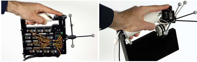
Figure 13: Devices used in the evaluation. (left) TextureTouch and (right) a modified NormalTouch controller, used for the NormalTouch interface, the VibroTactile interface (using an Xbox vibration motor), and the VisualOnly interface that tracked the user’s finger without haptic feedback.
