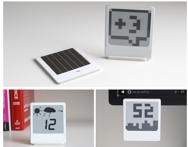
Figure 1. Our prototype ultra-low power displays (3 mm thick) combine an e-paper display with photovoltaic energy harvesting and Bluetooth LE wireless communications. The Post-it note form factor facilitates quick and versatile deployment. The photovoltaic panel is mounted on the rear of the unit (top) enabling the display to be deployed on a desktop (bottom left), attached to a monitor bezel (bottom right) or stuck to a window. We have built both segmented and dot-matrix style displays.
