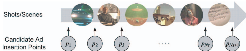
Fig. 7. Candidate ad insertion point detection in [79], [80]. Suppose there are N_s shot or scene boundaries in a video sequence, then the number of candidate points is N_s + 1 (including the beginning and the end of the video), each boundary indicating one candidate insertion point.
