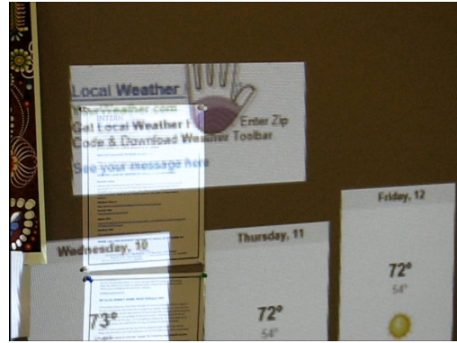
Fig. 8: SURROUNDWEB maps natural gestures to mouse events. Here, the user uses a standard “push” gesture to tell SURROUNDWEB to inject a click event into the web application.
