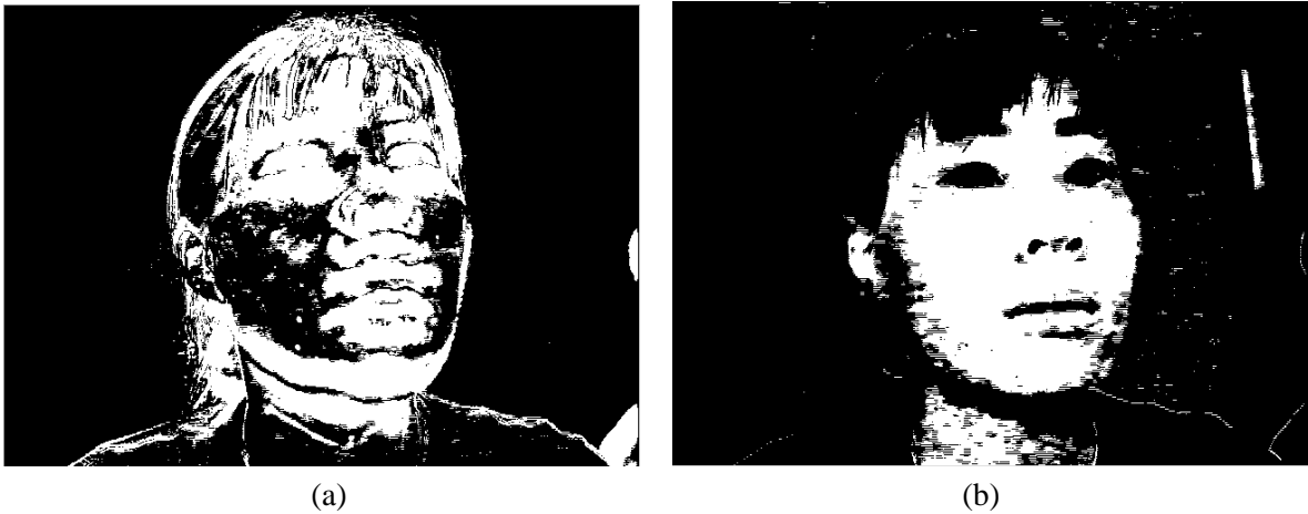
Figure 4: (a) Mask obtained by subtracting images (black pixels are considered as background); (b) Mask obtained by using a face skin color model (white pixels are considered as face skin).
