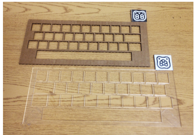
Figure 2. QWERTY keyboard touchplates in different materials. Touchplate is flipped upside-down so that the tag can be seen. Top: Cardboard cut by a laser cutter. Bottom: Clear acrylic cut by a laser cutter. Touchplates can also be cut by hand or 3D-printed.
