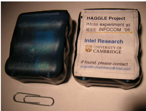
Figure 2: iMotes packaged for the experiment.
