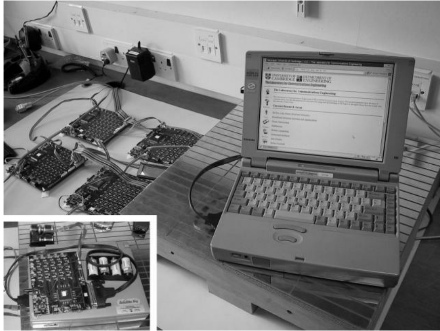
Figure 1: A notebook PC on the prototype Networked Surface (inset back of notebook)
