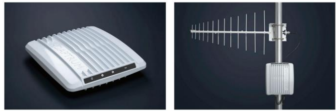
Fig. 2. The Adaptrum Radio ARCS 2.0. It measures 8.5 x 7.5 x 1.5 in
