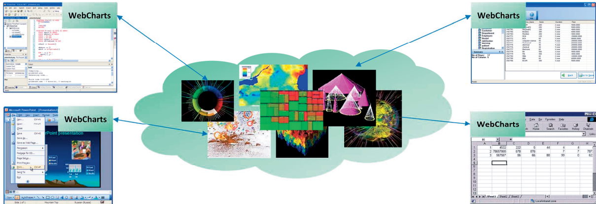
Figure 1: The WebCharts framework accommodates multiple types of visualizations, embedded in multiple types of applications. In this figure, four different host applications (around the outside) each dynamically add any WebCharts enabled visualization available on the web (center).
