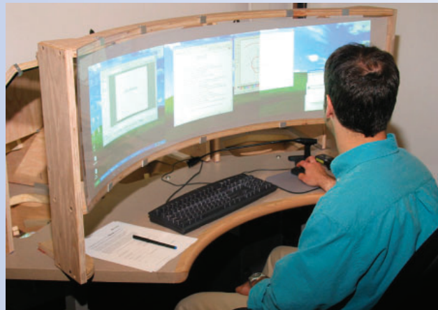
A DSharp multiprojector display.
