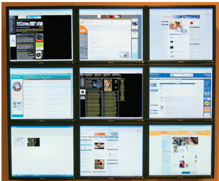
9 SimulBrowser. The technology shows how large displays enhance everyday activities, such as Web searching. Here, SimulBrowser shows search results in eight monitors, and selected pages in the ninth (lower left).
