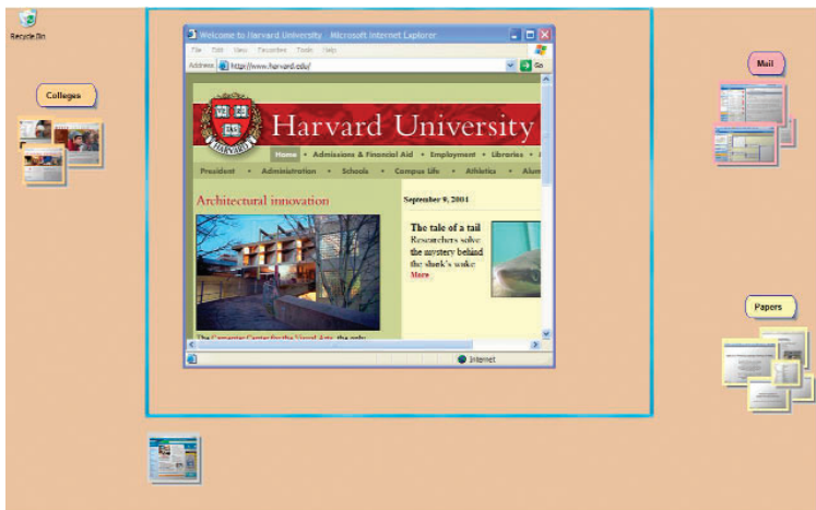
8 This Scalable Fabric example shows three task clusters in the periphery. By using the periphery, Scalable Fabric leverages the user's spatial memory and visual-recognition memory to aid task recognition.
