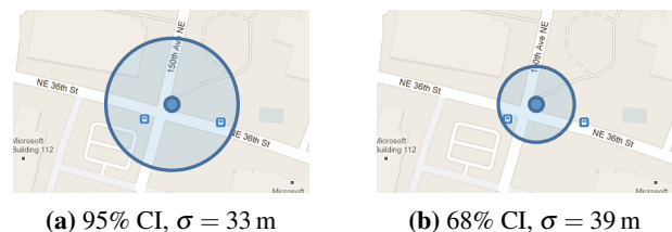
Figure 2. GPS samples at the same location on two smartphone platforms. Although smaller circles appear more accurate, the WP sample in (a) is actually more accurate.
