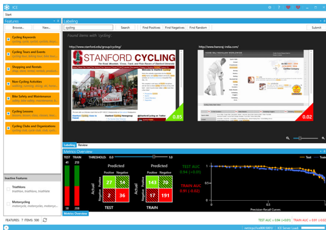
Figure 3. The ICE interface with traditional performance metrics used in machine learning (bottom panel). Users interactively label data in the labeling area (top right) and modify features in the featuring area (left). ICE automatically trains a model as a user supplies labels and features and displays its current performance in the panel at the bottom.
