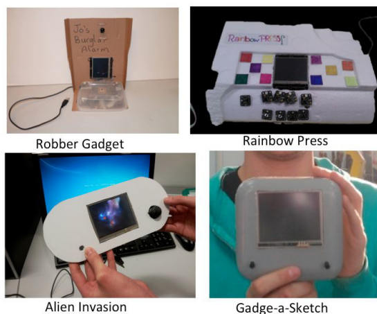
Figure 7: Examples of devices created by students with .NET Gadgeteer: “Robber Gadget” takes a picture of a burglar when a precious item is taken off the sensor platform; “Rainbow Press” is a reaction game; “Alien Invasion” is a shooting game; “Gadge-a-sketch” is a drawing device.
