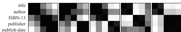
Figure 6: An illustration of the layout matrix A for five websites from the book vertical. The darker the matrix element, the closer the corresponding attributes in rendering.
