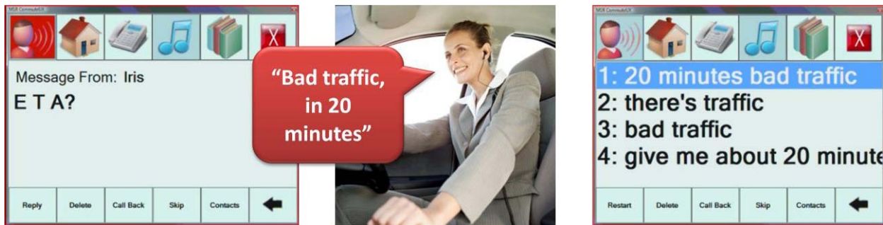
Figure 1. Screenshots of a multimodal automotive infotainment system for SMS replies which utilizes voice search to match empirically derived response templates.
