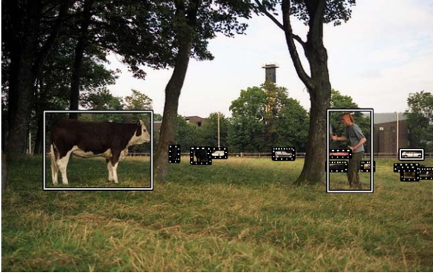
Fig. 3 Example of the “difficult” annotation. Objects shown dashed have been marked difficult, and are excluded from the evaluation. Note that the judgement of difficulty is not solely by object size—the distant car on the right of the image is included in the evaluation
