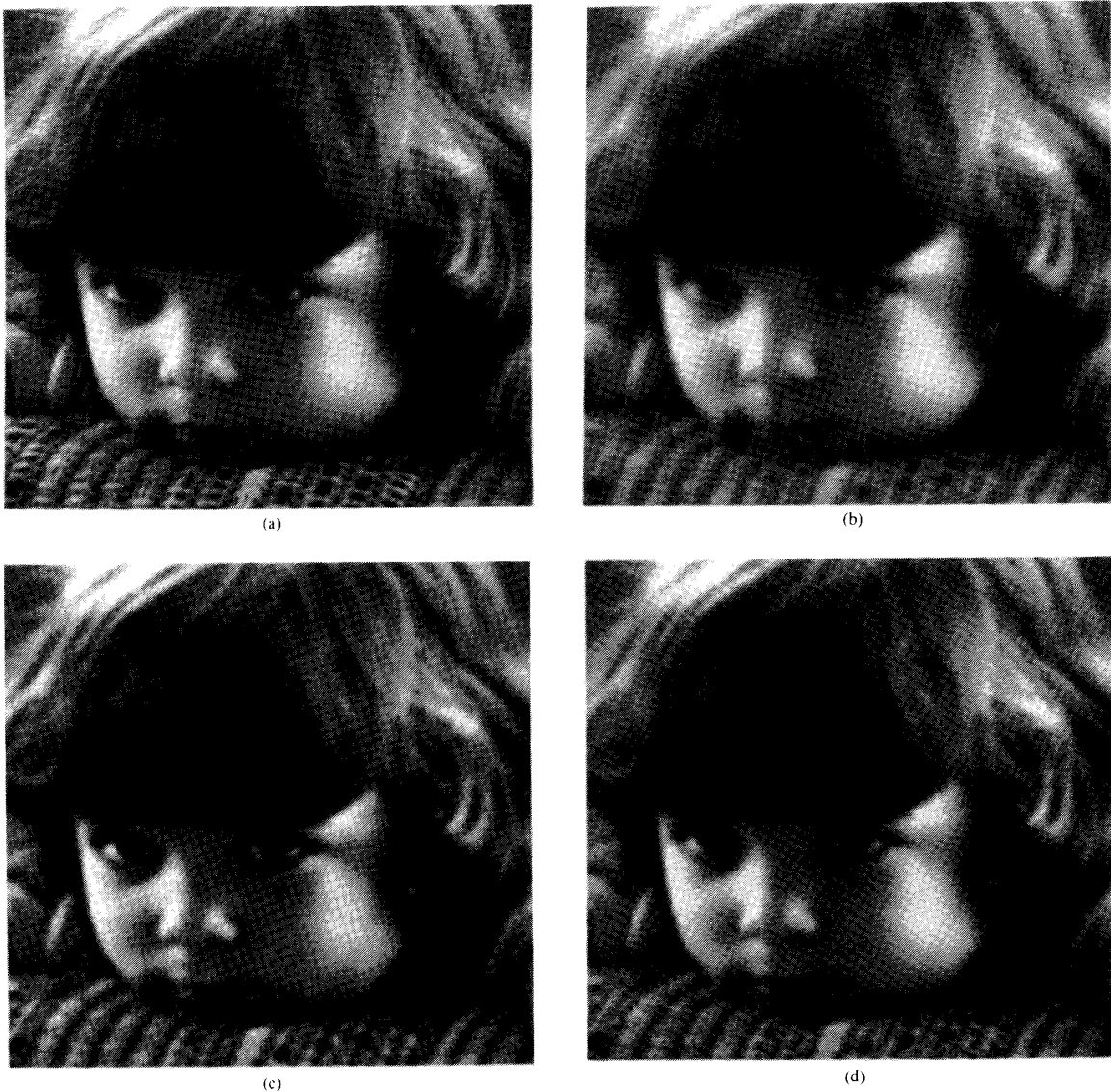
Fig. 3. (a) Original "KID" image, 256 \times 240 pixels, 8 bits/pixel. (b) "KID" processed with the linear prefilter and cubic convolution postfilter of Fig. 2(a) and (b), respectively; rms error = 19.3 percent. (c) "KID" processed with the Parks-McClellan prefilter and Oetken-Parks-Schüssler postfilter of Fig. 2(c) and (d), respectively; rms error = 13.7 percent. (d) "KID" processed with the mean-square-optimal pre- and postfilters of Fig. 2(e) and (f), respectively; rms error = 11.3 percent.
