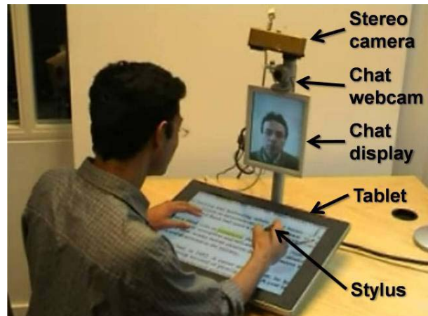
Figure 1: The C-Slate hardware setup comprising of a top-down stereo camera attached to a large tablet workspace, with a video conferencing display at eye-level to the user.
