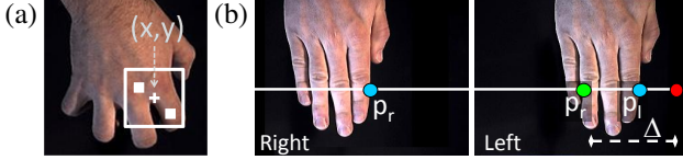
Figure 5. Visual features. (a) An example for a possible test in a decision tree. The test is applied to the pixel marked with the cross and the difference between two randomly selected pixels chosen within a bounding box of 50 \times 50 pixels is compared to two thresholds. (b) For a pair of corresponding pixels p_l and p_r from a stereo image pair the disparity d is computed as d = p_l - p_r .
