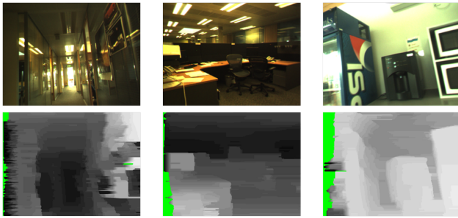
Fig. 4. Incorporating depth features. (Top row) Images of a corridor, cubicle space and kitchen, respectively. (Bottom row) Corresponding disparity maps computed using the dense stereo algorithm in [3].
