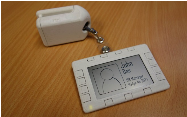
Figure 1. Prototype interactive badge and associated belt clip.
