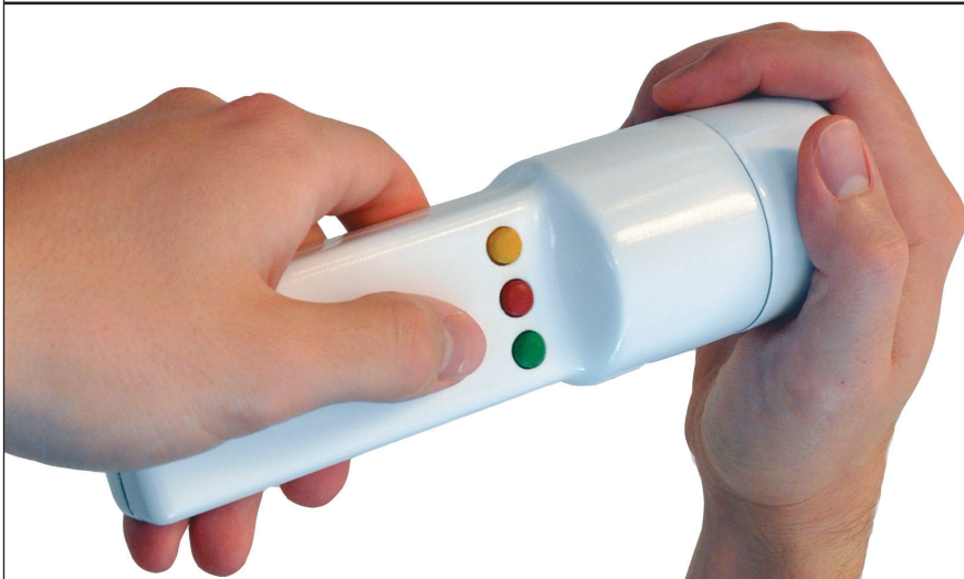
Figure 3. The Peppermill is an interaction-powered user interface device that can be used to control a TV. Rotating the Peppermill clockwise with the red button pressed turns up the volume, and with the green button pressed increments the channel.
