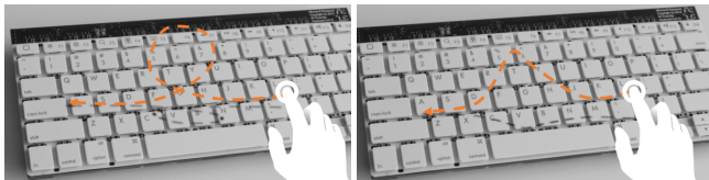
Figure 10. Dynamic hover gestures. Part of the gesture trajectory is performed in narrow band above the keyboard.
