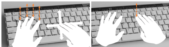
Figure 9. Micro-hover gestures. Hands remain in home position while typing or resting. Quick lifts off fingers triggers different commands.
