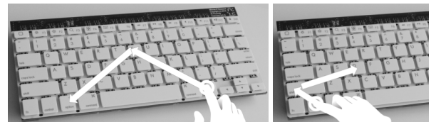
Figure 8. On-Keyboard shapes. Shape drawing to perform discrete commands. Physical keyboard as landmark may help as mnemonic aide in gesture memorization.
