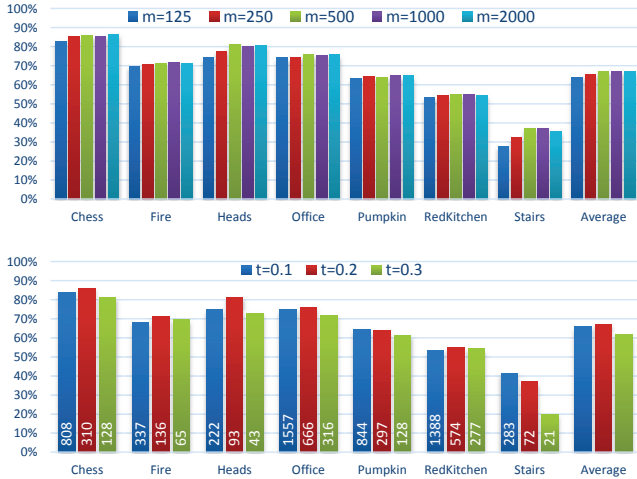
Figure 5: Parameter evaluation: Relocalization performance when varying the number of ferns m (top graph) and changing the keyframe acceptance threshold t (bottom graph). Initially increasing the number of ferns improves performance, which levels off after m=500 . The threshold t influences the number (in white) and density of keyframes. Optimal coverage is obtained with t=0.2 (see Fig. 2 for an example).
