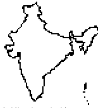
Figure 6. Thresholding the resized image produces a binary image.
