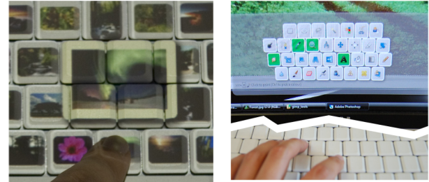
(b) Content-preview of clips. (c) Preview of finger positions on a virtual on-screen keyboard
