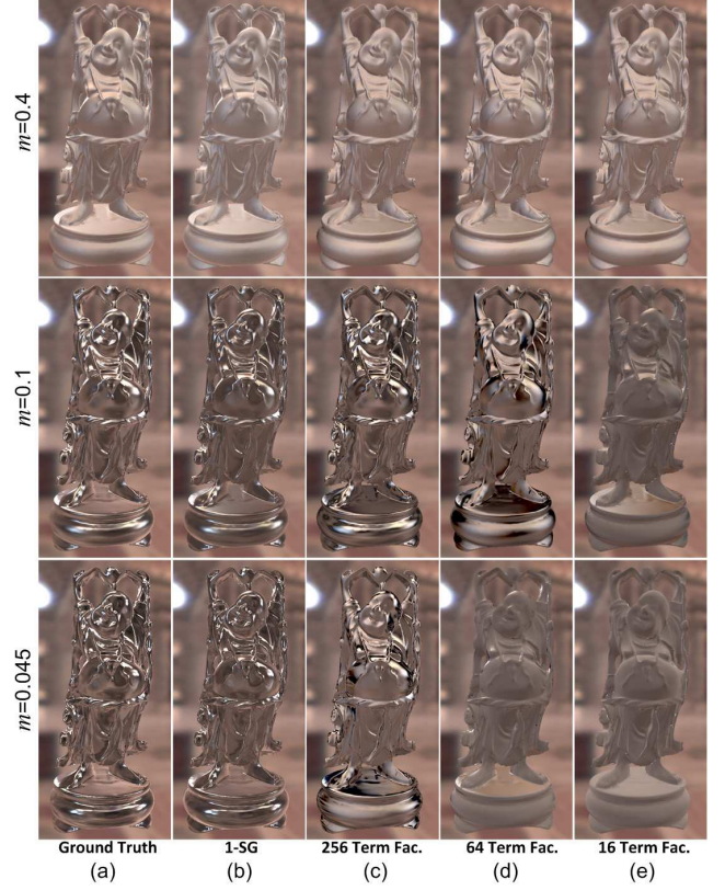
Figure 4: Rendering comparison with parametric, isotropic BRDFs: (a) ground truth, (b) single-lobe SG model, and BRDF factorization with (c) 256 terms, (d) 64 term, and (e) 16 terms.
