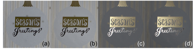
Figure 4: SVBRDF fitting on a measured example from [Lawrence et al. 2006]. Two light/view settings are shown: (a,c) original, (b,d) our approximation with 2 SG lobes per pixel.
