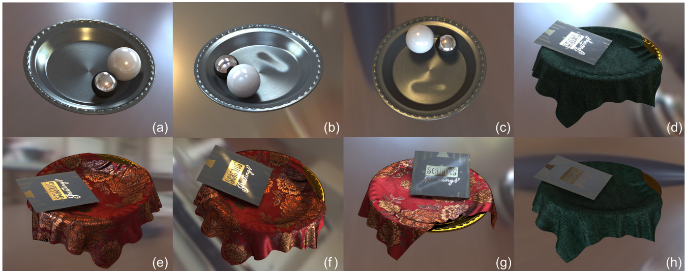
Figure 12: Rendering results with anisotropic BRDF models. (a) Dishes and balls using Ashikhmin-Shirley model. (b,c) Painted tangent rotation. (d-h) Measured cloth (5-lobe SG) and greeting card (2-lobe SG). (f,g) Painted SG warp suggesting wet paint.
