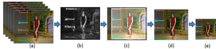
Fig. 1. Retargeting system overview: scale-space spatiotemporal saliency map (b) is calculated from consecutive n video frames (a). A minimal information loss cropping window with the target aspect ratio is identified via smooth saliency tracking (c), and the cropped image (d) is isotropically scaled to the target display (e). This example retargets 352 \times 288 images to 100 \times 90 .
