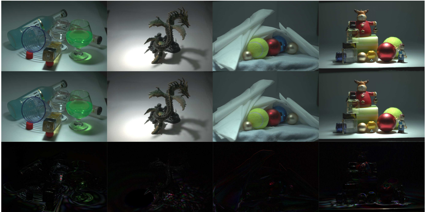
Figure 12: Visual comparison of relighting results. Images in the first row are captured from each scene as illuminated by a point light source that is not used when acquiring images for the light transport matrix reconstruction. Images in the second row are rendered from the reconstructed light transport matrices of the scenes under the same lighting condition. The third row shows the difference images, with their intensities scaled up by a factor of 10.
