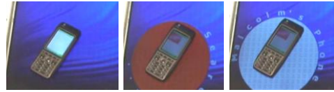
Figure 6: Synchronizing an untagged mobile device with the ThinSight display using the device's camera and Bluetooth.
