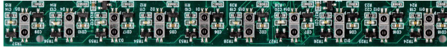
Figure 3: The SideSight sensor PCB. The ten IR proximity sensors are clearly visible. Note: photodiodes are on the top, emitters directly underneath.
