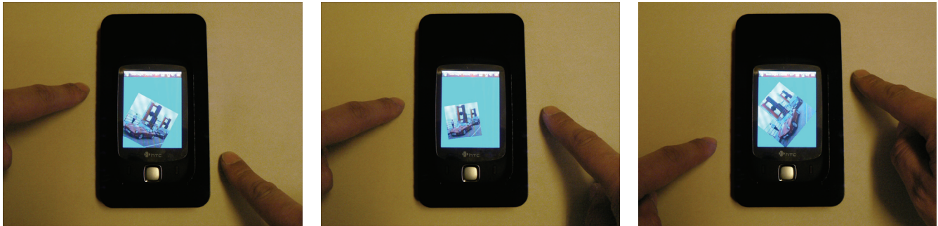
Figure 1: SideSight supports virtual multi-“touch” interactions around the body of a small mobile device. Optical sensors positioned along each edge of the device allow fingers to be sensed as they approach the device from the sides. In the example depicted, the device is resting on a flat surface, and fingers touching the surface on either side of the device are sensed to provide multi-touch input. As the left-hand finger is moved down and the right-hand one moved up (looking through the sequences of images from left to right), the photo on the display is rotated anticlockwise.
