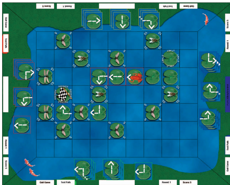
9 The Sides tabletop computer game requires a group of children to form a path enabling a frog to travel from the start lily pad to the end lily pad. Along the way, if this path intersects with insects, the group scores bonus points. The distribution of arrow pieces forces all four users to cooperate in order to form a valid path. Buttons along each side of the table enable users to vote on key game interactions (for example, testing the path or quitting).
