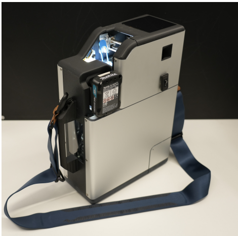
Figure 2: Prototype fiber and transceiver cleaning robot.
