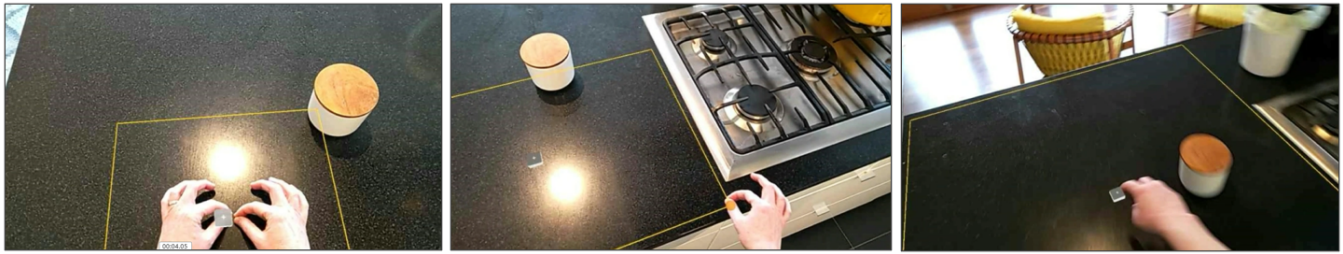
Figure 3: Interactive approach to defining tracking regions. Left: Tracking region is created with a double-pinch gesture; region is displayed in mixed reality as a rectangular yellow hologram. Center: Size of the tracking region modified by pinching and moving one of its corners. Right: Position of the tracking region confirmed by push of virtual [+] button.
