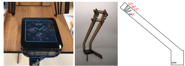
Figure 2: Left: The Sony Smartwatch 3 used in all three studies. Middle: Our custom-made study stand. Right: The angles we used in the study represented on a sketch of our study stand.
