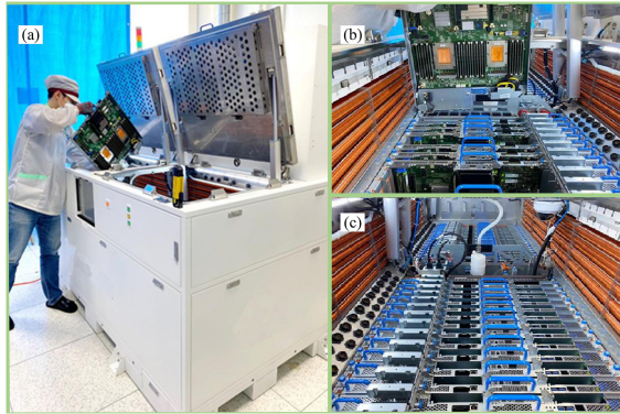
FIGURE 2. Large 2PIC tank prototype.
