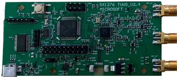
FIGURE 3. FarmBeats IoT radio utilizes TV white spaces for long-range communication.
