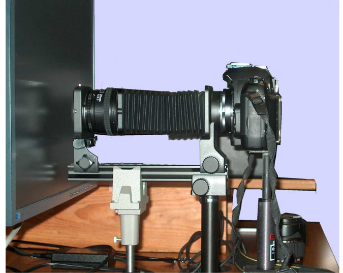
Fig. 1. Nikon D100 digital camera with a customized lens and light baffle to measure the spatial distribution of light intensity produced by red, green, blue, and white pixels. The lens is a 20-mm focal length objective placed in the reversed direction. In this position, the lens magnifies the pixels by a factor of 10 on the camera sensor.
