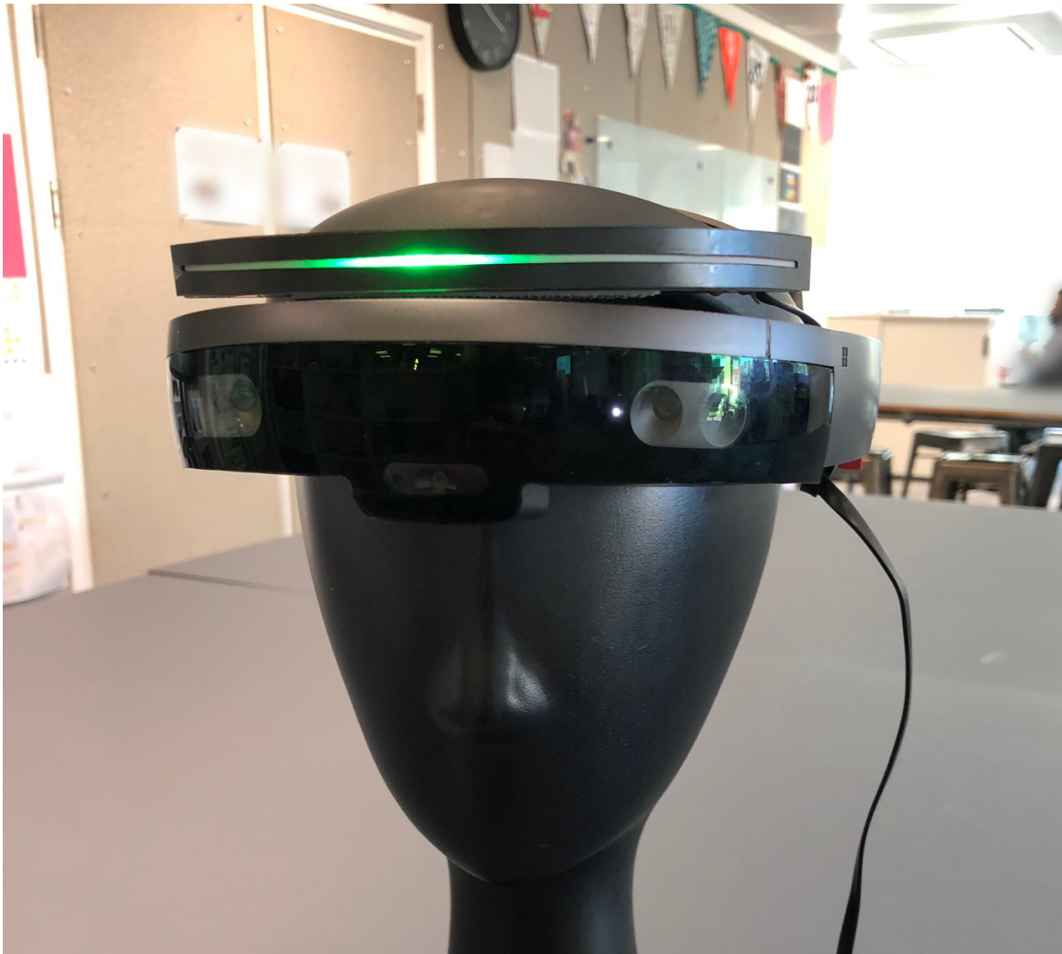
Figure 2: Modified HoloLens device with external LED display.
