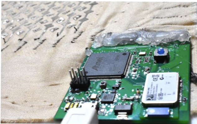
Figure 5. Capacitive sensing board. The button and header pins are used for debugging.
