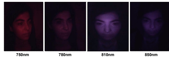
Fig. 9. NIR imagery with different Near-IR LED wavelengths.
