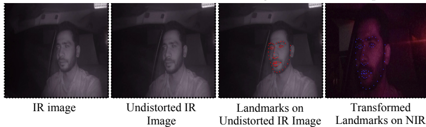
Fig. 14. Distorted and undistorted IR images along with label translated NIR image.
